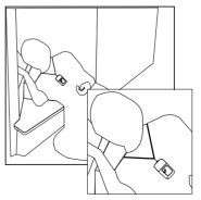
For best results we recommend the using the neck cord provided to allow the keyfob to hang around the neck. Placing the keyfob in a pocket may reduce the effectiveness of the shock sensor.
